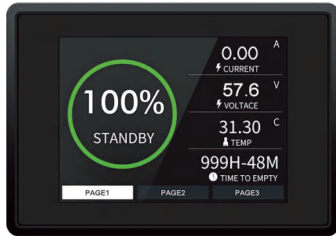
100%Capacity/SOC 0.00A Charge/Discharge Current
