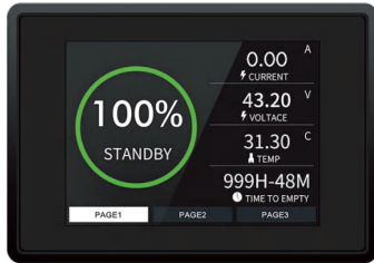
100%Capacity/SOC 0.00A Charge/Discharge Current
