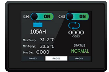
DSG Discharge State CHG charge State
